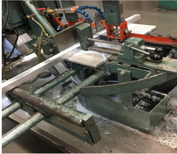
Figure 20: Cutting the Aluminum Frame
