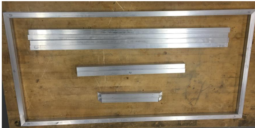
Figure 21: Fully. Cut Aluminum Frame for Hood
