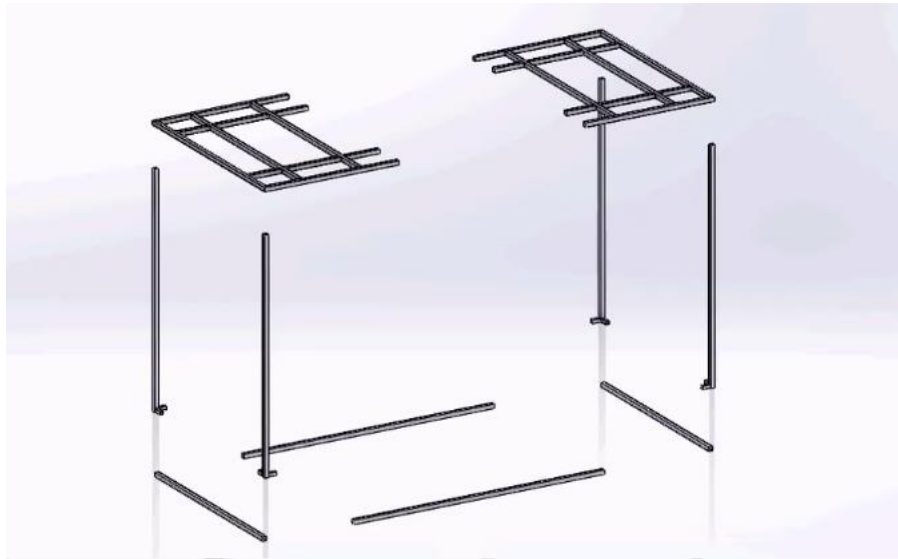
Figure 25: Disassembled Steel Frame
