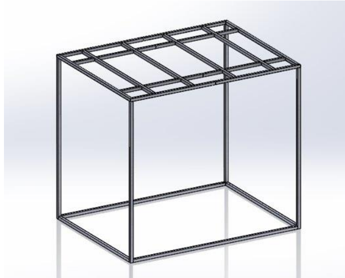
Figure 24: Redesigned Steel Frame for Room
